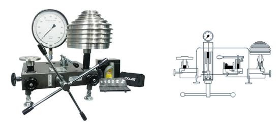
Models of DW 30 series are provided with 2 free piston assemblies for giving Low Pressure range with smaller steps and High Pressure range with larger steps in a single instrument with substantial cost saving. The ratio of areas of LP and HP Free Pistons is generally 10:1. Ratio of 5:1 or 20:1 can also be provided.
