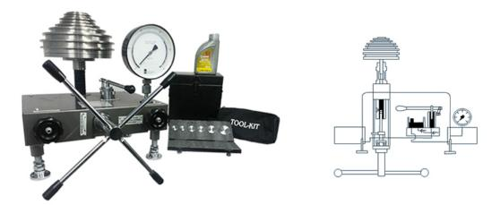
Models of DW 20 and DW 30 series are provided with a lever operated Priming Pump also giving continuous oil delivery for filling up large gauges or even external piping. It is capable of developing 10% of instrument range and with isolating valves at both ends. If form a unique closed circuit for effective air removal.
