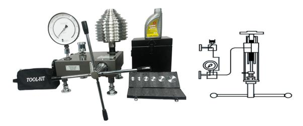
Models of DW 10 series are provided with one large capacity screw pump and a removable oil reservoir with isolating valve in a simple line circuit permitting effective air removal.
