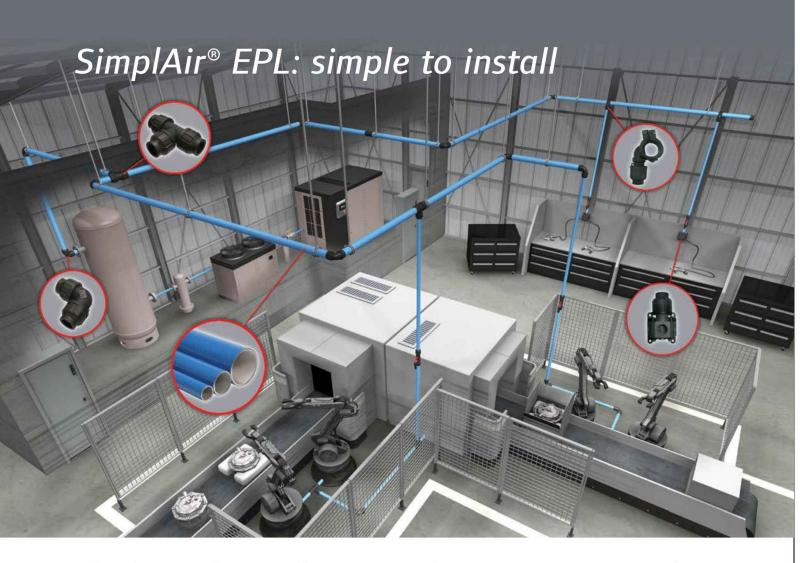
With a modular design and easy-to-assemble components, the SimplAir® EPL piping system empowers you to easily plan and adapt your distribution piping network to the needs of your production environment.
