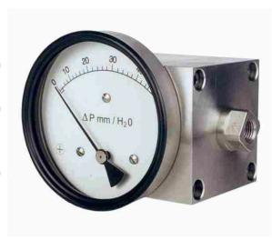
Manometer India manufactures quality differential pressure instruments designed to measure the difference in pressure between two points in a system and show it on a single dial instrument. A magnetic movement senses the differential pressure. The instruments has separate pressure and indicating chambers.
