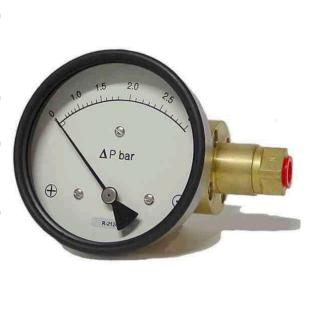
Manometer India manufactures quality differential pressure instruments designed to measure the difference in pressure between two points in a system and show it on a single dial instrument. A magnetic movement senses the differential pressure. The instruments has separate pressure and indicating chambers.
